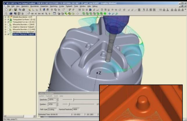
Above - All the machining moves have lead in/out arcs to maintain a smooth machine motion. The cutting moves are also smooth, flowing profiles without sudden changes of direction
