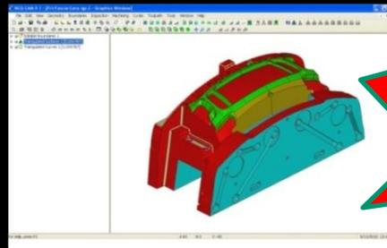
*Above – Core side of an injection mould tool for a car facia*
