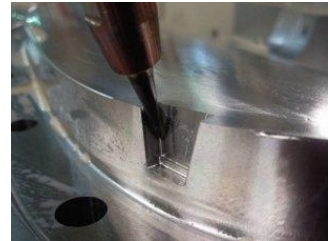
Right - Using 3+2 with small cutters to minimise spark erosion
