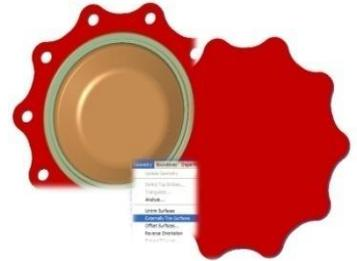
**NCG CAM** also has the ability to create internal fillets, this can in some instances allow a more flowing toolpath. Planar patches can also be created to cap or protect areas if needed.
