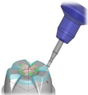
Tool axis control allows the user to have some control of how the tool tilts:
