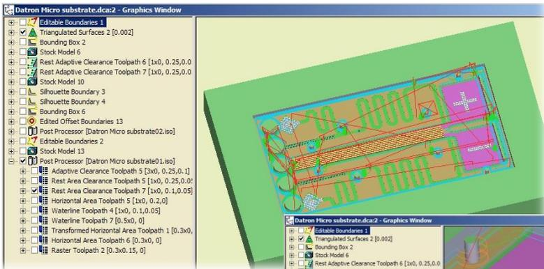
*Right- Close up of the part showing the detail and waterline passes.*
